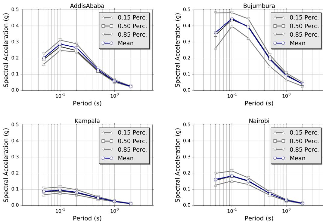
**Fig. 12** Mean and quantile Uniform Hazard Spectra (UHS) computed at the four selected African capitals for 10% probability of exceedance in 50 years (475 year return period). It is worth noting how the mean and the 0.5 percentile curves are generally in good agreement and overlapping, with the only noticeable exception of Addis Ababa in the 0.1s to 0.2s spectral period range.
