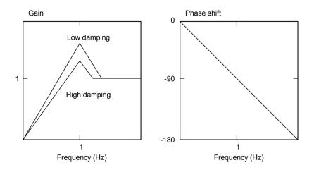
**Figure 2.3** The amplitude and phase response of a mechanical seismometer. The curves are derived qualitatively. The free period of the seismometer is 1.0 s. The phase shift is in degrees. For the gain, a curve for low and high damping is shown. For the exact curves, see Figure 2.4.
