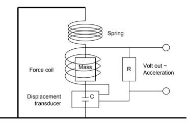
**Figure 1.4** Simplified principle behind Force Balanced Accelerometer. The displacement transducer normally uses a capacitor *C*, whose capacitance varies with the displacement of the mass. A current, proportional to the displacement transducer output, will force the mass to remain stationary relative to the frame.
