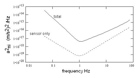
**Figure 2.37** The same as in Figure 2.36, but in this case the noise is specified as an equivalent ground acceleration noise, that is, the ground acceleration that would produce the voltage output noise represented in Figure 2.36.
