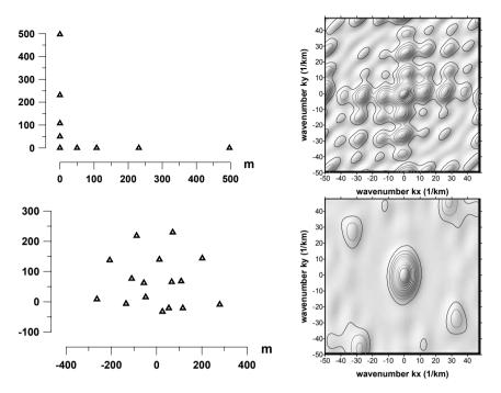
**Figure 9.5 (cont.)** Different examples of small aperture array shapes and their transfer functions. A bi-axial one, with a sharp response but some degree of multiple aliasing, and a random array derived from the semicircular one with random spatial deviations, which shows a good sharp response, improving the resolution along the *ky*-axis.
