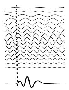
**Figure 6.6** Sum of harmonic functions (top) that become the wavelet seen at the bottom. Reprinted from *Modern Global Seismology* by Lay and Wallace (1995), p. 177; copyright (1995), with permission of Elsevier.
