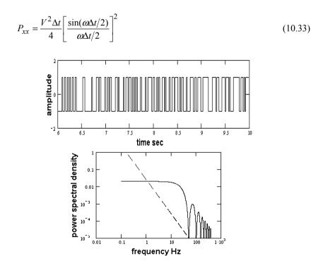
**Figure 10.20** A section of a pseudo-random binary signal (PRBS) (upper) and its power spectral density (lower, solid trace), compared with the PSD of a step with the same amplitude (dashed line). The PRBS presents a flat level until a corner frequency that may be as high as desired, depending on the generator clock interval.
