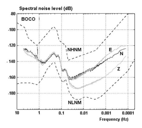
**Figure 3.4** The Peterson noise curves and noise spectral level for the IRIS station BOCO. The noise level is in dB relative to  $1 \text{ (ms}^{-2})^2$ /Hz. The Peterson high and low noise models are shown with dashed lines. The noise spectra are shown for all 3 components. Note the lower noise level for the vertical (Z) component (note that x - axis represents decreasing frequency). Figure modified from FDSN station book, http://www.fdsn.org/FDSNpubs.htm.
