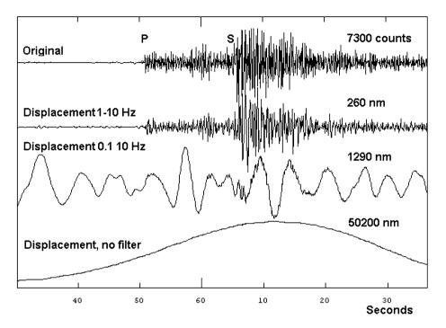
**Figure 6.9** Instrument correction in different filter bands. The top trace is the original recording of a small earthquake with a 1 Hz seismometer. The 3 bottom traces have been converted to displacement with different filters. The amplitudes to the right are maximum amplitudes.
