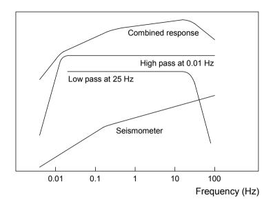
**Figure 6.13** Combining response functions. The figure shows the displacement response function of the seismometer and the amplitude response functions of the two filters. Both scales are logarithmic. The y-axis is arbitrary.
