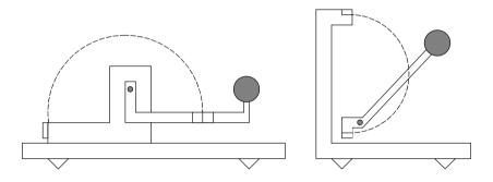
**Figure 2.17** Leaf spring astatic suspensions. The figure to the left shows a vertical seismometer and to the right an oblique axis seismometer. Redrawn from Figure 5.10 by E. Wielandt in NMSOP, Vol. 1, Bormann (Ed.), 2002; copyright granted by IASPEI.
