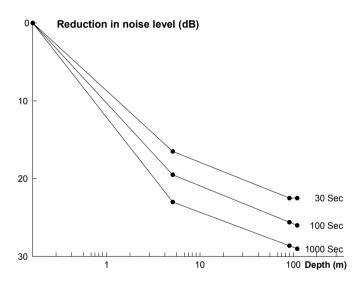
**Figure 7.9** Horizontal noise attenuation (dB, spectral acceleration density) as a function of depth and period. Modified from Fig. 7.59 by L.G. Holcomb in NMSOP, Vol.1, Bormann (Ed.), 2002; copyright granted by IASPEI.
