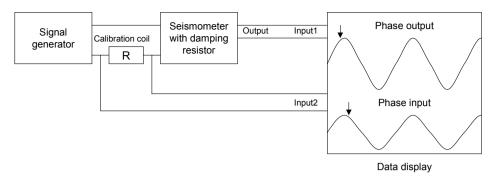
**Figure 10.8** Calibration for frequency response with a seismometer with a calibration coil. The resistor R is used to have simple way of measuring the current through the calibration coil by measuring the voltage over R. The recorder shows the input and output signals which have different amplitude and phase. The output has a positive phase shift relative to the input.
