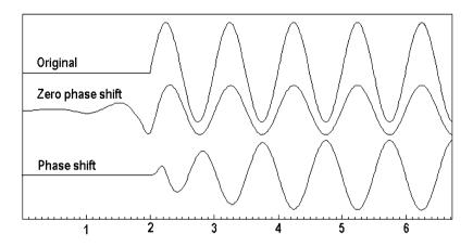
**Figure 6.12** The effect of using filters on a signal with a sharp onset. The signal is a 1 Hz sine wave with an onset at 2 s (top trace). The middle trace shows the signal filtered with a zero phase shift Butterworth filter while the bottom trace shows the signal filtered with a Butterworth filter with a phase shift. Both filters are band pass with corners at 1 and 5 Hz.
