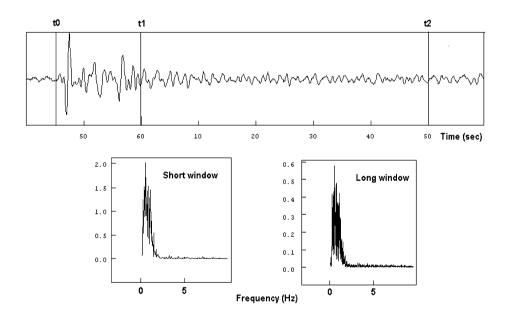
**Figure 6.8** The signal (top) is a teleseismic P-phase recorded using a short period seismometer. Below is shown the amplitude spectra of the short window (t0-t1) and the long window (t0-t2). The scales on the axes are linear. Note that the short window has a higher level than the long window. Also note that the frequency estimates are much closer together for the long window.
