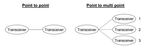
**Figure 8.13** Point to point or point to multi point system. To the left is shown the traditionally point to point system while to the right is shown a point to multipoint system. Here only one frequency is used to communicate to 3 stations, one at a time. A solid line shows that there is a continuous communication.
