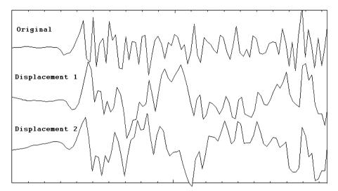
**Figure 2. 5** Effect of using the wrong instrument correction. The top trace shows the P-phase of a local earthquake. The distance between the tics is 0.1 s. Displacement 1 trace shows the displacement in the frequency band 1-20 Hz using the 'correct' equation while the trace Displacement 2 shows how the displacement trace looks with the "wrong" correction for phase.
