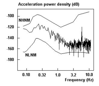
**Figure 3.5** Noise power density spectrum of the raw signal seen in Figure 3.1, top trace. The acceleration power is in dB relative to 1  $(m/s^2)^2/Hz$ . The limits of the Peterson noise model are indicated (NHNM and NLNM). The spectrum has not been smoothed.
