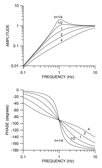
**Figure 2.4** The amplitude and phase response functions for a seismometer with a natural frequency of 1 Hz. Curves for various level of damping h are shown.
