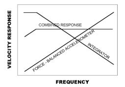
**Figure 2.21** Simplified response elements of a velocity broadband sensor showing log-log velocity response of gain versus frequency. The idealized response of each element is shown (all slopes are 1 or -1), as well as the combined response.
