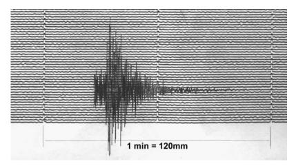
**Figure 5.3** An example of an analog recording from a SP recorder. The figure shows part of a seismogram. The time marks are 60 s apart.
