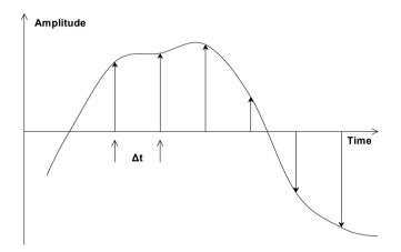
**Figure 4.1** The analog to digital conversion process. The arrows show the location and values (amplitudes) of the samples and the signal is thus approximated with a sequence of numbers available at time intervals  $\Delta t$ .
