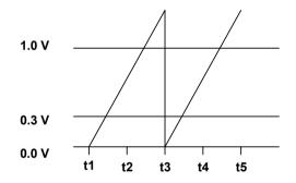
Figure 4.5 Improving dynamic range by oversampling in the presence of noise, see text.
