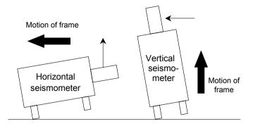
**Figure 10.6** Polarity test. By tilting the sensor in the direction of the thin arrow, the seismometer mass moves only in the direction of the thick arrow. For the horizontal component, the tilt should be made in a time shorter than the natural period; otherwise the relative motion might be in the opposite direction, due to the weight of the mass, which will naturally go down.
