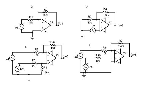
**Figure a.11** Several linear applications of the *op amp* as amplifier. a) Inverting amplifier. The voltage gain in this example is -10. b) Non inverting amplifier. The gain is (1+10)=11. c) Differential amplifier. The output voltage is ten times the difference v3-v4. d) A summing amplifier. The output in this example is  $v_{04}=-10(v_5+v_6)$ .
