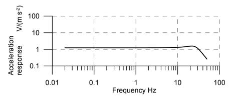
Figure 2.27 Frequency response of filtered FBA.
