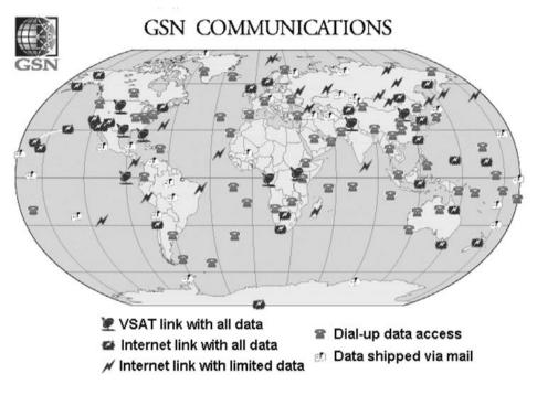
**Figure 8.23** Communication to GSN stations in 2001. VSAT is a satellite connection. VSAT and internet have real time connections and potentially all data can be downloaded, while the dial up stations only transmit a limited amount of data. Figure from www.iris.washington.edu.
