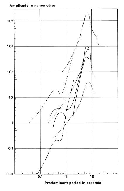
**Figure 3.3** Noise curves in a rural environment. The 3 dotted lines correspond to the maximum, mean and minimum levels published by Brune and Oliver (1959), the dashed lines give two extreme examples observed in the US and the full line curves give the limits of fluctuation of seismic noise at a European station on bedrock in a populated area 15 km away from heavy traffic (figure from Wilmore, 1979).
