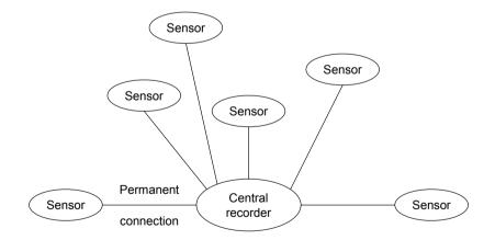
**Figure 8.5** A physical seismic network. The sensors are connected to a central recorder through a permanent physical connection like a wire or radio link. In this example, transmission is analog and digitization takes place centrally, but the ADC could also have been placed with the sensor and transmission would then be digital.
