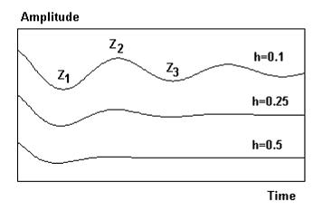
**Figure 2.10** Effect of damping on the signal. The sensor has been given some initial positive displacement and then left swinging freely. The damping constant is *h*. The extreme amplitude values are  $z_1$ ,  $z_2$  and  $z_3$ . It is seen that for a damping of 0.5, there is little over swing.
