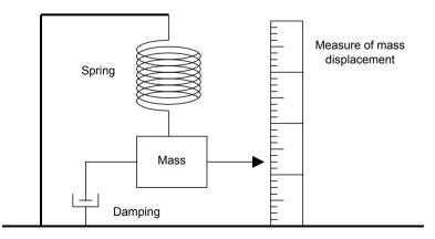
Figure 1.3 Principle behind the inertial seismometer. The damping of the motion can be mechanical, but is usually electro-magnetic.
