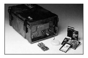
**Figure 5.14**. Example of a recorder made specifically for strong motion, the Kinemetrics Etna. The round white box in front of the recorder is the GPS antenna and the PCMCIA cards are seen to the right. From Kinemetrics home page www.kinemetrics.com.
