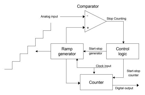
Figure 4.4 Ramp ADC, see text.
