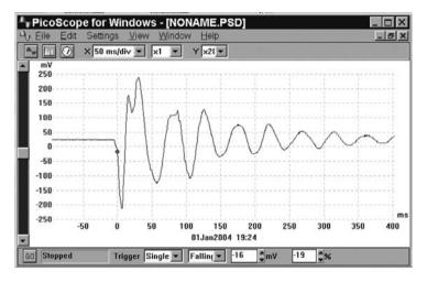
**Figure a.8** An example of a virtual oscilloscope made with a laptop using a cheap module of data acquisition (from Pico Technology, www.picotech.com) and the accompanying program. Almost all the controls normally available in a real oscilloscope are present.
