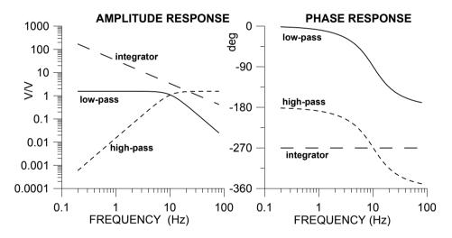
**Figure a.14** Amplitude (left) and phase (right) response of the low-pass second order filter of Figure a.13b (solid), the integrator of Figure a.13a (long dashes) and a second order high pass filter (short dashes). Note the similarity of the latter with the mechanical seismometer response for ground displacement. The phase response of the integrator is –270 degrees instead of –90 because the sign inversion of the circuit in Figure a.13a.
