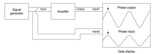
**Figure 10.21** Basic setup for testing and calibrating an amplifier. The data display can be a recorder for which the calibration is known. The display shows that the output signal has a positive phase shift (leads the input).
