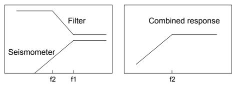
**Figure 2.22** Enhancing frequency response by inverse filtering. The response functions are shown as log gain versus log frequency. The seismometer has corner frequency *f1* and the special filter corner frequencies *f1* and *f2* (left). To the right is seen the combined response.
