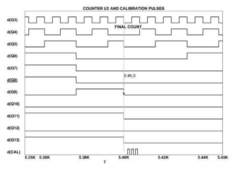
**Figure a.18** The waveforms at several outputs of the counter U2 and the calibration sequence, immediately before and after the final count (5400). The calibration sequence is triggered by this state.
