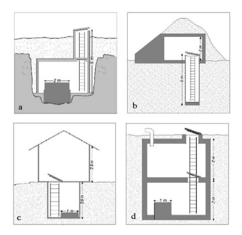
**Figure 7.7** Example of BB vaults from the GEOFON network. a) Underground bunker vault for remote recording, b) Wide and shallow borehole type, c) and d) Simple bunker construction. Note that b – d allow onsite recording since there is a separate recording room. Copied from Fig. 7.55 by W. Hanka in NMSOP, Vol.1, Bormann (Ed.), 2002; copyright granted by IASPEI.
