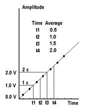
**Figure 4.6** Digitization of a linearly increasing signal. The ADC has levels 0, 1 and 2 V corresponding to counts(c) 0,1 and 2. The running average of 4 samples represented by times t1..t4 is given in the table under 'Average'.
