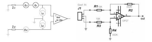
**Figure 2.35** Left: A noise model of an instrumentation differential amplifier.  $e_n$  represents the internal noise voltage referred to the input,  $e_{s1}$  and  $e_{s2}$  are voltage noise sources associated to the signal sources, and  $i_{n1}$  and  $i_{n2}$  are current noise sources associated to each amplifier input. Right: A typical differential seismic amplifier, whose noise is estimated in the example below.
