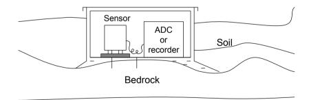
**Figure 7.4** Typical installation of a 3 component station and optional equipment. The box is a common aluminum transport box. Part of the bottom has been cut out and is the bottom has been covered by cement, which has been fixed to the bedrock with a few pieces of iron drilled in. Insulation has been put in around the sides and in the lid.
