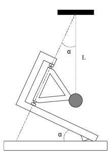
**Figure 2.13** Principle of the garden gate pendulum. The tilt angle is exaggerated. A string pendulum must have length L to have the same period, so at a small angle  $\alpha$ , L becomes very large. Redrawn from Figure 5.8 by E. Wielandt, in NMSOP, Vol. 1, Bormann (Ed.), 2002; copyright granted by IASPEI.
