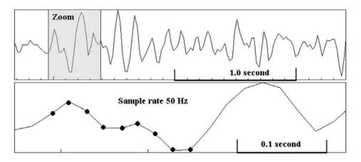
**Figure 1.5** Example of a digitized earthquake signal. The top trace shows the signal with a low time resolution and the bottom trace, the zoom window with a high resolution. In the zoom window, the discrete samples are clearly seen. The sampled points are indicated with black dots.
