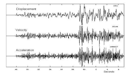
**Figure 2.8** A signal from a magnitude 3 earthquake recorded with a 1 Hz seismometer. The 3 traces show displacement, velocity and acceleration, respectively, in the frequency band 0.3-20 Hz. The numbers on top of the traces at the right hand side are the maximum amplitudes in nm, nm/s and nm/s<sup>2</sup>, respectively.
