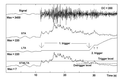
**Figure 5.7** The seismic trigger. Top trace is the original signal; the second trace, the *STA*; the third trace *LTA* and the last trace the *STA/LTA* ratio. The *STA* window is 0.4 s and the *LTA* window is 50 s. The trigger ratio is 3 and the de-trigger ratio 2.
