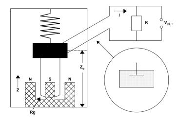
**Figure 2. 6** A model of an electromagnetic sensor. The coil resistance is  $R_g$ , the damping resistor is R and the voltage output is  $V_{out}$ . The dashpot damping has been replaced by the damping from the coil moving in the magnetic field (redrawn and modified from Scherbaum, 2001, with kind permission of Kluwer Academic Publishers).
