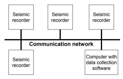
**Figure 8.6** A virtual seismic network. The thick line is the communication network, which can have many physical solutions. The data collection computer can collect data from some or all of the recorders connected to the network provided that it knows the protocol used by the recorder. Both types of seismic networks might result in the same kind of output although the virtual network will deliver data with a larger time delay than most of the advanced physical networks.
