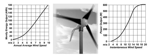
**Figure 7.16** The Air 403 wind generator. To the left is shown the monthly energy output as a function of average wind speed. To the right is shown the power output as a function of the instantaneous wind speed (Figure modified from Southwest Windpower, www.windenergy.com).
