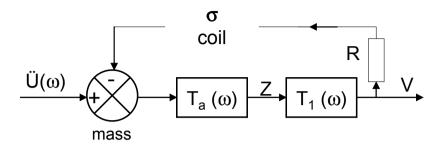
Figure 2.25 Block schematics of a FBA system.
