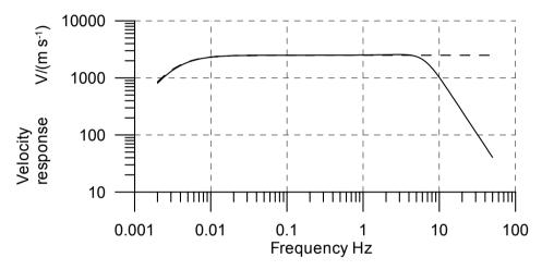
Figure 2.29 Frequency response of a BB system
