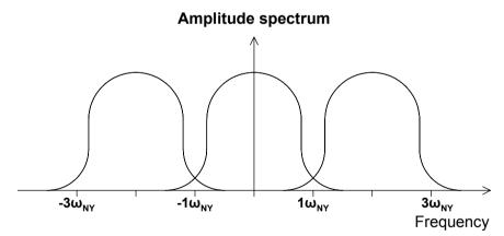
**Figure 6.7** The aliasing effect in the spectral domain. The Nyquist frequency is  $\omega_{NY}$  and it is seen that the spectrum repeats itself for each  $2\omega_{NY}$  and that there is overlap when the signal frequency is larger than  $\omega_{NY}$ .
