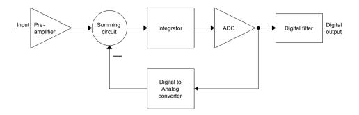
**Figure 4.8** Simplified overview of a sigma-delta ADC. The signal from the ADC is converted back to analog with the digital to analog converter (DAC). The summing circuit subtracts the ADC signal from the input signal. The digital converter ADC, the integrator and the digital to analog converter are all synchronized and controlled by a logic circuit (not shown).
