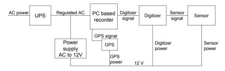
**Figure 7.14** Station based on custom made components and AC operation. UPS stands for uninterruptible power supply. The connections are shown as single wires for simplicity.
