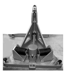
**Figure 2.14** A typical horizontal long period seismometer made by Sprengnether. The two black cylinders seen at each side are the magnets and the coils are moving inside with the mass in the center. Leveling is done with the 3 screws at the corners of the base plate. Once the horizontal leveling is done (front screws), the back screw is used to adjust the period. The base plate side length is 63 cm and the weight 45 kg.
