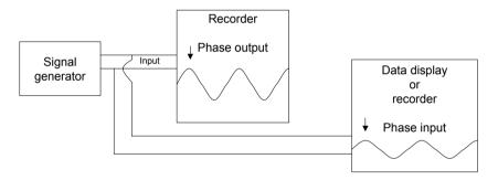
**Figure 10.22** Basic setup for testing and calibrating a recorder. The data display can be a recorder for which the calibration is known. Note that the output signal is recorded with the recorder itself since the output is the digitized signal.
