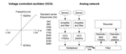
**Figure 8.12** Analog transmission using frequency modulation. To the left is shown the VCO and standard frequencies used. The figure shows the linear relationship between the voltage input and frequency out for a carrier frequency of 1700 Hz. To the left is shown a network of two stations using two different carrier frequencies which are summed in the multiplexer, separated in the filter and demodulated in the demodulator.
