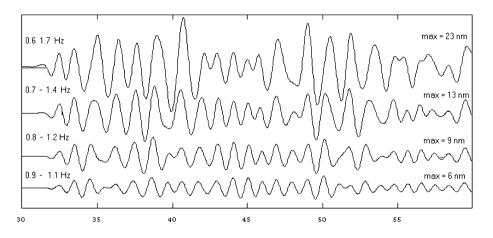
**Figure 3.2** The signal from Figure 3.1 band pass filtered with different filter widths. The signals have been corrected for instrument response to show displacement. The maximum amplitude in nm is shown to the right on top of the traces.
