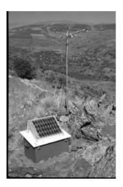
**Figure 7.15** A small 12 W mono-crystalline solar panel mounted on top of the case of a temporary seismic station. Both sides of the panel are light sensitive, so the roof of the case is white-painted to reflect the diffuse radiation to the rear side of the panel.
