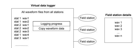
**Figure 8.10** Simple virtual data logger. The field station (right) has a waveform file for each detected event (wav 1, wav 2 etc). The virtual data logger (left) simply copies all the waveform files from all stations to a directory on the central computer (stat1 wave1 etc). Further processing is done manually.
