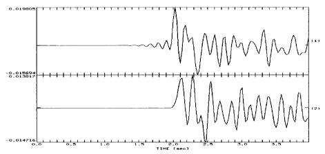
**Figure 6.10**. Precursory effect of a FIR filter. The top trace shows the original recorded signal, and the bottom trace the corrected signal. Reprinted from Scherbaum (2001), with kind permission of Kluwer Academic Publishers.
