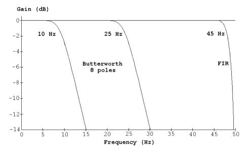
**Figure 4.11** A FIR filter compared to Butterworth filters. The FIR filter has a gain of -150 dB at the 50 Hz Nyquist frequency, while the 10 and 25 Hz Butterworth filters have gains of -42 and -112 dB respectively.
