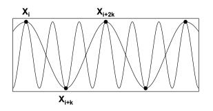
**Figure 5.8** The difference filter. A 1 Hz and a 3 Hz signal is shown. Subtracting sample  $x_{i+k}$  from  $x_i$  gives constructive interference using the 1 Hz signal sampled at 2 samples/second or multiple of this, while subtraction  $x_{i+2k}$  from  $x_i$  gives destructive interference. The same is true for the 3 Hz signal.
