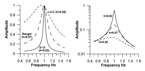
**Figure 10.3**. The spectral amplitudes of the calibration pulses with the sensor output open, plotted in a narrow band centered on the sensor natural frequency. Left: The amplitude scale is linear and the amplitude of each trace has been normalized with respect to its maximum. Right: The amplitude scale is logarithmic and the factor  $a_0G$  is taken as unity.
