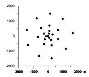
**Figure 9.4** ARCES is a small aperture array with 25 stations covering four concentric circles. The diameter of the external ring is about 3 km. The radial spacing of the stations is not uniform in order to deal with different wavelength.
