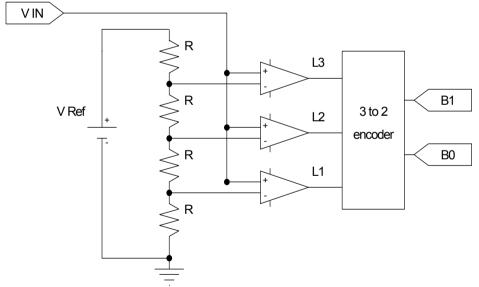
**Figure 4.2** Flash ADC. *Vin* is the signal to be digitized, *R* are resistors of equal size, *Vref* is a reference voltage. The circuits at right are comparators. L1 to L3 are the direct outputs of the comparators, which are coded to a two bit output, B0 and B2, since only four values are possible. This example is actually a two-bit digitizer (see later).
