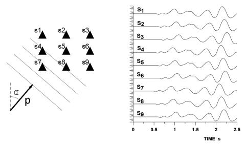
**Figure 9.3** Left: A plane wavefront arrives with apparent slowness *p* to a rectangular shaped array (the intersection of the wavefront with the surface, where the array is installed, is shown). The angle  $\alpha$  with respect to North defines the ray arrival azimuth. Right: The waveforms recorded are ideally identical, except for the relative delays. In practice, they present differences due to the added noise and to the local ground heterogeneity.
