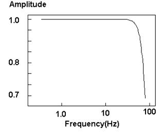
**Figure 6.14** Response curve corresponding to the last 3 poles and the normalization constant as given in Table 6.2 for the seismometer in stage 1. Both axis are logarithmic.
