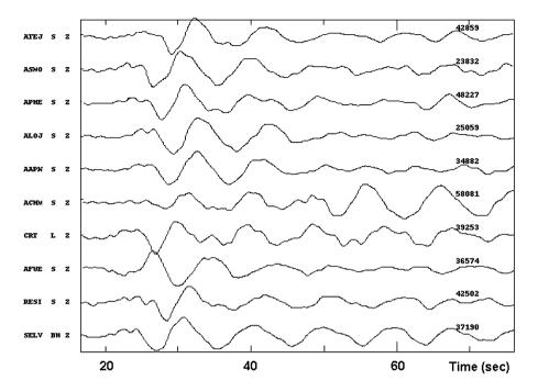
**Figure 10.7** A distant earthquake recorded on a microearthquake network (200 km diameter) with eight SP stations (S Z), one LP (L Z) and one BB (BH Z). The traces have been filtered in the frequency band 0.1 to 1 Hz and converted to displacement. The numbers to the right are maximum displacement in nm. Note that station AFUE clearly has inverted polarity.
