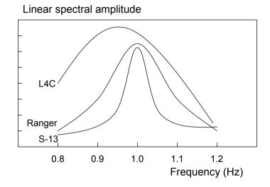
**Figure 10.2** Spectral analysis of the signals in Figure 10.1. A 100 s time window has been used to get sufficient frequency resolution. The three spectra are plotted with linear amplitude; however, the amplitude scaling for each one is different.
