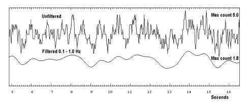
**Figure 4.7** Unfiltered and filtered record of seismic background noise in a residential area in Western Norway on a hard rock site. The recording is made with a 4.5 Hz geophone and a 16-bit ADC at a sample rate of 50 Hz (GeoSIG GBV116). The filter is an 8-pole Butterworth filter with zero phase shift.
