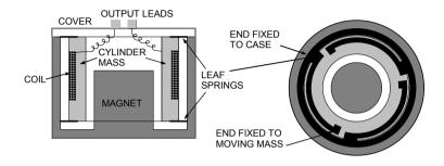
**Figure 2.42** Typical construction of a geophone. Note the leaf spring suspension. The magnet is fixed to the case and the coil moves with the mass.
