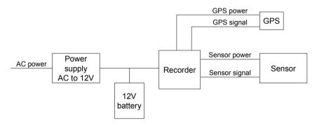
Figure 7.13 Self contained recorder running off main power. The connections are shown as single wires for simplicity.
