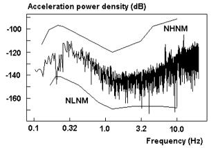
**Figure 7.2** Noise spectrum of the first one-minute window from the record in Figure 7.1. The vertical scale is dB relative to 1  $(m/s^2)^2/Hz$ . The Peterson noise models are shown (NHNM and NLNM, Chapter 3).
