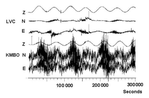
**Figure 7.10** Records from two different VLP stations. The earth tides are clearly seen on all records. Note the higher noise on horizontal components than on vertical components (modified from Fig. 7.53 by W. Hanka in NMSOP, Vol.1, Bormann (Ed.), 2002; copyright granted by IASPEI.
