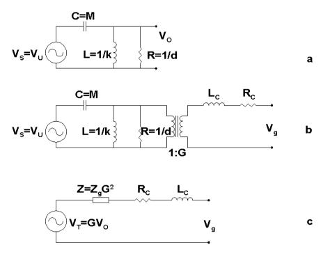
**Figure 2.34** Equivalent circuit of a sensor. a) Mechanical sensor. b) The same with a velocity transducer. A transformer is used for coupling the equivalent circuit to the real charge, see text. c) The circuit of b where the virtual part (the transformer and everything on its left) has been replaced by its Thévenin equivalent.
