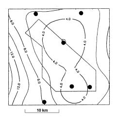
Figure 8.4 Isolines of the uncertainty of epicenter determination in km for a small local network, figure modified from Trnkoczy & Zivzic (1992), by permission of E.C.G.S.
