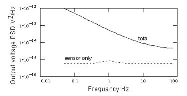
**Figure 2.36** The output voltage noise PSD at the output of the amplifier due to the sensor noise and the total noise including the amplifier noise: It is clear that this latter is the most relevant contribution.
