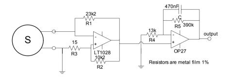
**Figure 2.30** Typical feedback system for extending the response of a velocity sensor. The component values shown were calculated for a 4.5 Hz Mark L15 of 380 ohm.
