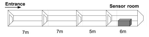
**Figure 7.8** Horizontal tunnel construction with different chambers used by USGS IRIS. The total length of the tunnel is 25 m (redrawn from Fig. 7.52 by W. Hanka in NMSOP, Vol.1, Bormann (Ed.), 2002; copyright granted by IASPEI.
