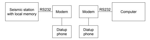
**Figure 8.20** Manual dial up to a seismic station for data inspection and/or download. The computer dialing can be any type of computer with a terminal emulator program like Hyperterminal in Windows.
