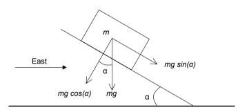
Figure 10.15 Tilting an accelerometer to determine generator constant. It is assumed that the sensor horizontal direction is towards East.
