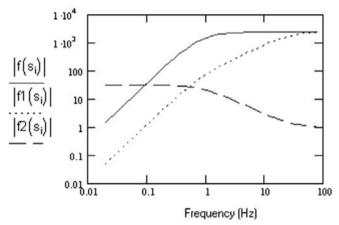
**Figure 2.31** Velocity response of an overdamped and amplified sensor (dots), the equalizing filter (dash) and the combined response (solid). Note that the new corner frequency is 1 Hz. Vertical axis unit is  $V/(m \cdot s^{-1})$ .
