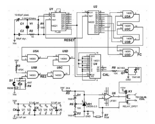
**Figure a.17** A circuit to generate a sequence of three calibration pulses every twelve hours. U1 has a crystal oscillator and a 24-stage counter, U2 divides the frequency further and together with the logic about U3 and U5, provides two pulses per day. U4 generates then the three pulse sequence. The voltage reference VR1 and the opamp U6 form a current source connected to the sensor coil by K1, controlled by the pulses. See text.
