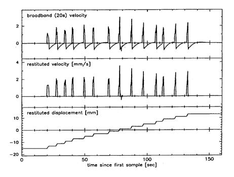
**Figure 10.14** Absolute calibration of a 20 STS1-BB using a milling machine. The sensor was moved 14 steps of 2 mm each. The top trace shows the original recording. The middle trace shows the pure velocity record (de-trending and corrected for response) while the bottom trace shows the displacement obtained by integrating the middle trace. Reproduced from Figure 5.29 by E. Wielandt in NMSOP, Vol. 1, Bormann, (Ed.), 2002; copyright granted by IASPEI.
