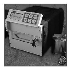
**Figure 5.11**. The Lennartz MARSliteHD recorder. Below the display is seen the 3.5" extractable hard disk. The model with magneto-optical recording is less than half the size (bottom part missing). From Lennartz home page, www.lennarz-electronic.de.
