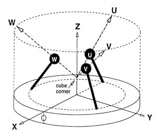
Figure 2.44 The triaxial geometry of the STS-2 seismometer. The oblique components are W, V and U. From Figure 5.13 bye E. Wielandt, in NMSOP, Vol. 1, Bormann (Ed.), 2002; copyright granted by IASPEI.
