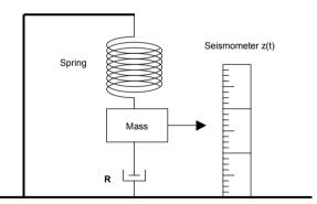
Figure 2.1 A mechanical inertial seismometer. R is a dash pot.
