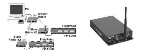
**Figure 8.14** A Spread Spectrum central station communicates to two data acquisition systems (left). Right is shown the Data-Linc Spread Spectrum radio modem model SRM6000 (RS232) or model SMR6000E (Ethernet). The range is 40 km with whip antenna and 55 km with Yagi antenna (40 and 50 km respectively for model E). For more details, see Table 8.2. Figure from www.data-linc.com, by permission of Linc Technology Corporation/dba Data-Linc Group.
