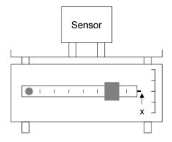
**Figure 10.13** Moving a sensor a controlled distance vertically with a mechanical balance. The ratio between the motion at x (where we can measure it) and on the balance table can be determined by placing a mass m1 at x that will balance a mass m2 at on the balance table. The ratio of the two motions is then m1/m2. Redrawn from Figure 5.30 by E. Wielandt in NMSOP, Vol. 1, Bormann, (Ed.), 2002; copyright granted by IASPEI.
