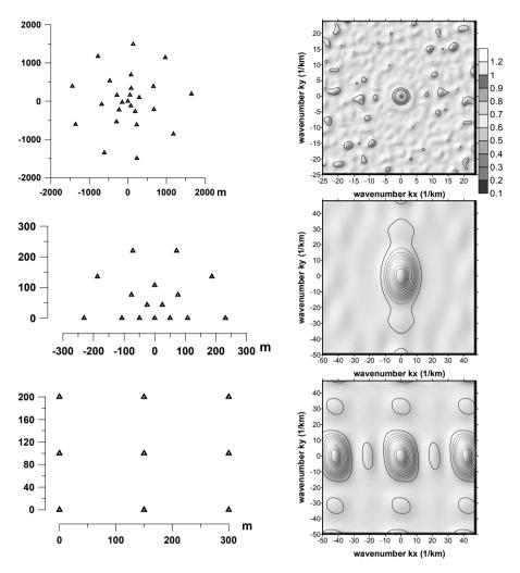
**Figure 9.5** Different examples of small aperture array shapes and their transfer functions. Top, the array ARCES, mentioned above, with 25 stations and a diameter of 3 km, has a sharp almost ideal response. Next, there is a semicircular array, a rectangular one with a response showing spatial aliasing (ghost peaks).
