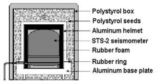
**Figure 7.6** GEOFON BB installation. There is a thick (3 cm) aluminum base plate and a thinner aluminum helmet with a cylindrical foam rubber insert (redrawn from Fig. 7.50 by W. Hanka in NMSOP, Vol. 1, Bormann (Ed.), 2002; copyright granted by IASPEI.
