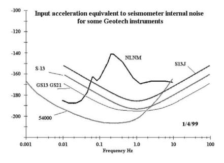
**Figure 2.40** Instrument sensitivity of several Geotech seismometers (Table 2.3 and 2.4) ranging from the short period S-13 to very broad band 54000 seismometer. The curves show input acceleration equivalent to sensor internal noise in dB relative to  $1(ms^{-2})^2/Hz$  (see also Chapter 3). NLNM is the Peterson New Low Noise Model (Peterson, 1993). Slightly modified from Geotech home page, www.geoinstr.com, with permission.
