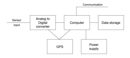
**Figure 5.6** Main units of a seismic recorder. There are no flow arrows between the units since all can have two way communications. The GPS can be connected to the digitizer or the recorder. The power supply may be common for all elements or each may have its own regulator, but usually the power source is unique (e.g. a battery).
