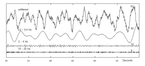
**Figure 3.1** Seismic noise in different filter bands at station MOL in the Norwegian National Seismic Network The short period station (1 Hz) is situated about 40 km from the North Sea and the unfiltered trace clearly shows the high level of low frequency noise (~0.3 Hz) generated by the sea. All traces are plotted with the same scale and the numbers to the right above the traces are the maximum amplitude in counts.
