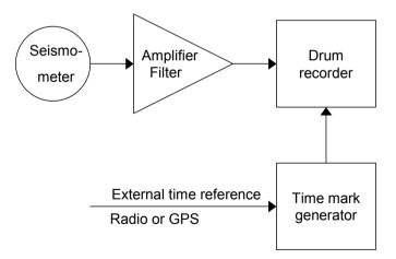
**Figure 5.2** A complete analog recorder. The time mark generator is an accurate real time clock which might be synchronized with an external time reference.
