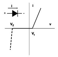
**Figure a.3** A piecewise linear model of the diode volt-ampere characteristic.  $v_t$  is the threshold voltage, below which the diode is not a conductor. For an inverse voltage  $v_z$  the current increases quickly with a small voltage increment (dashed line). There exist Zener diodes designed to operate in this zone as voltage references.
