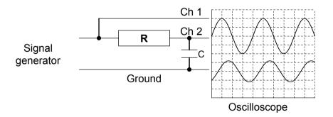
**Figure 6.4** Measuring the amplitude response function of an RC filter. The signal from a signal generator goes directly to channel 1 (Ch1) on the oscilloscope and to channel 2 (Ch2) through the filter so both input and output is measured.
