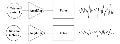
**Figure 10.12** Comparison of signals recorded from two different seismometers with the same recording equipment. The filters and amplifiers are identical and filter out signals below the seismometer natural frequency. The ratio of the output amplitudes (right) indicates the ratio of the sensor generator constants.
