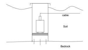
**Figure 7.3** Typical installation of a 1 Hz vertical seismometer. The sensor is inside a PVC tube with an airtight screw on the lid (standard sewage tube). There is cement at the bottom, which has been fixed to the bedrock with a few pieces of iron drilled in. The sensor is placed on a glass, ceramic or plastic plate.
