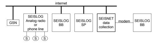
**Figure 8.26** Types of stations in the Norwegian National Seismic Network (NNSN). Nearly all stations are connected by internet (fixed or ISDN dial up). Abbreviations are: S: Seismic stations in a local network and GSN: Quanterra type GSN station.
