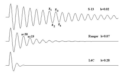
**Figure 10.1** Free swinging of three typical 1 Hz seismometers with different open circuit damping h. Traces have been generated synthetically. The decaying extremes (peak amplitudes) are labeled  $z_1$ ,  $z_2$  etc (top trace). On the middle trace, the amplitudes of two maximums following each other are given in an arbitrary scale.
