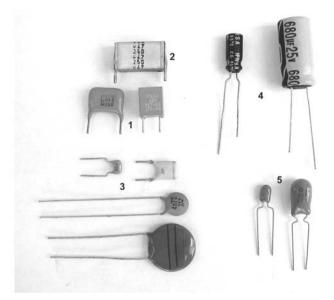
**Figure a.2** Capacitors made with several types of dielectrics. 1: Polyester types of medium capacity 10-1000nF. 2: Polycarbonate. 3: Ceramic disk or multilayer (low capacity, high frequency). 4: Electrolytic, high capacity. 5: Solid tantalum. 4 and 5 are polar capacitors and have a limited voltage range.
