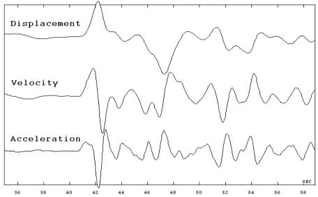
**Figure 6.11** A P-wave from a teleseismic event original recorded on the velocity trace. The two other traces show displacement and acceleration. Note that the polarity of the onset is the same on all 3 traces.
