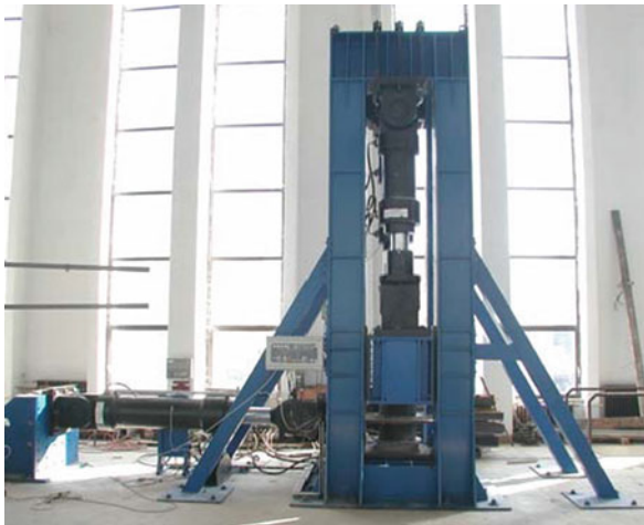
Fig. 17.16 Big two-componental testing machine
