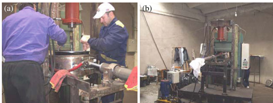
Fig. 17.15 Production of prototype large bearing: (a) assemblage of the shim plates and rubber sheets in the mold (b) curing process
